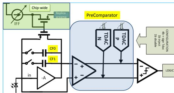
Figure 2: Block diagram of analog front-end.
