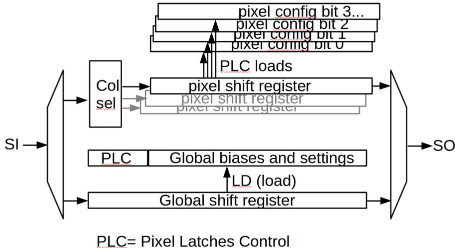
Figure 5: Configuration register data flow.
