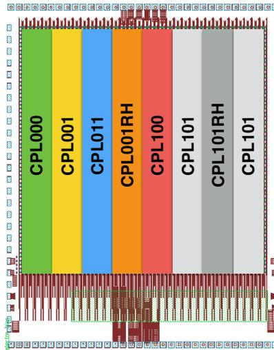
**Figure 4:** Illustration of analog FE column variants.
