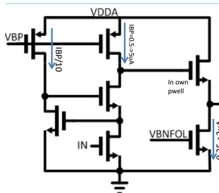
Figure 3: Pre-amplifier schematic.
