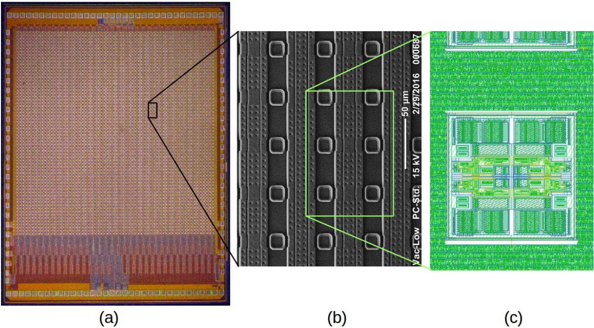
**Figure 1:** (a) Photograph of FE65-P2. References to bottom, top, left, and right throughout the text assume the orientation in this picture. (b) SEM micrograph showing detail with several bump pads on  $50\ \mu\text{m}$  pitch visible. The column power bus structure can also be seen. (c) layout detail showing an analog quad island surrounded by synthesized logic.
