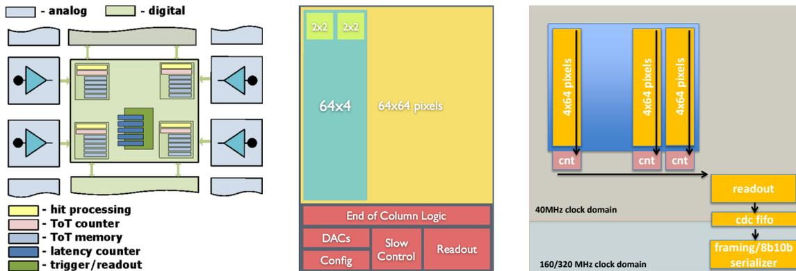
Figure 8: FE65-P2 digital layout and data flow.
